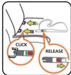
**STEP 1:** Press the ISOFIX release button and push the ISOFIX attachment forward. Do these step in both sides of the booster seat.
