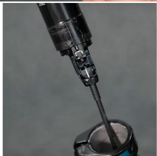
3. Once inserted, pull the cable through at the headtube
