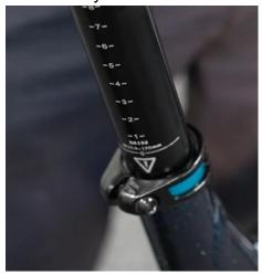
5. Check with the remote (located in the left side of the handle bar) if your seat post able to fully extended
